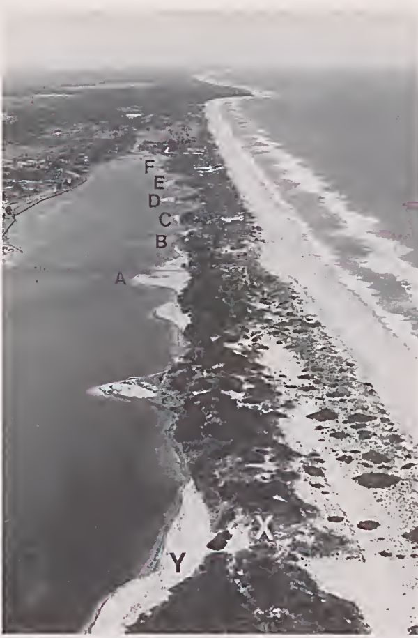
Fig. 9—The southern shoreline of Cunninghame Arm, Lakes Entrance, looking eastward to Red Bluff. Sand spits, formerly nourished by dunes spilling over the enclosing barrier (especially at X), and now augmented by dredged sand dumped on the shore (Y), are migrating eastwards. A to F are the features shown in Fig. 8.
